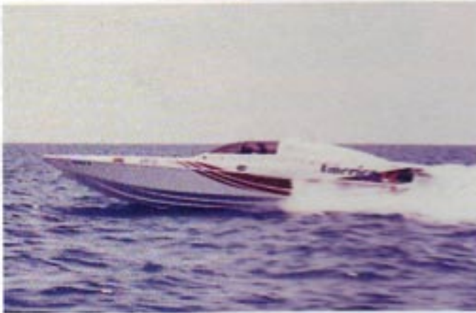
46' Cougar endurance race boat with triple Cat diesels, Arneson ASD 10 surface drives.
